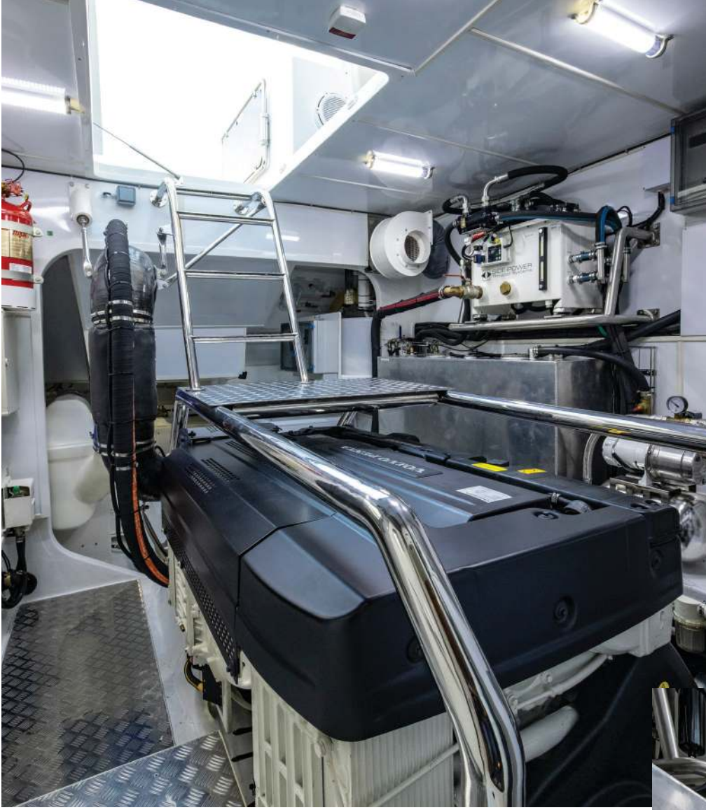
2X D13 1000 HP Volvo Penta Diesel Engines.
