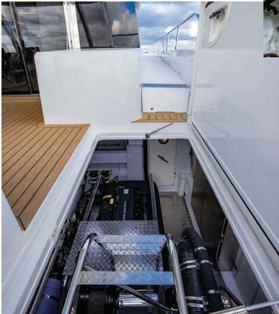
Engine Room Access Via Deck Hatch or Interior Water-Tight Door.
